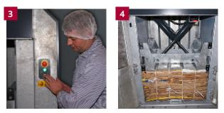
1 Compact your waste and eject the finished bale. 2 Remove and store the bale until collection. 3 The bale is ejected by a safe two-hand operation. 4 The cross cylinders ensure stable compression and a low overall height.
