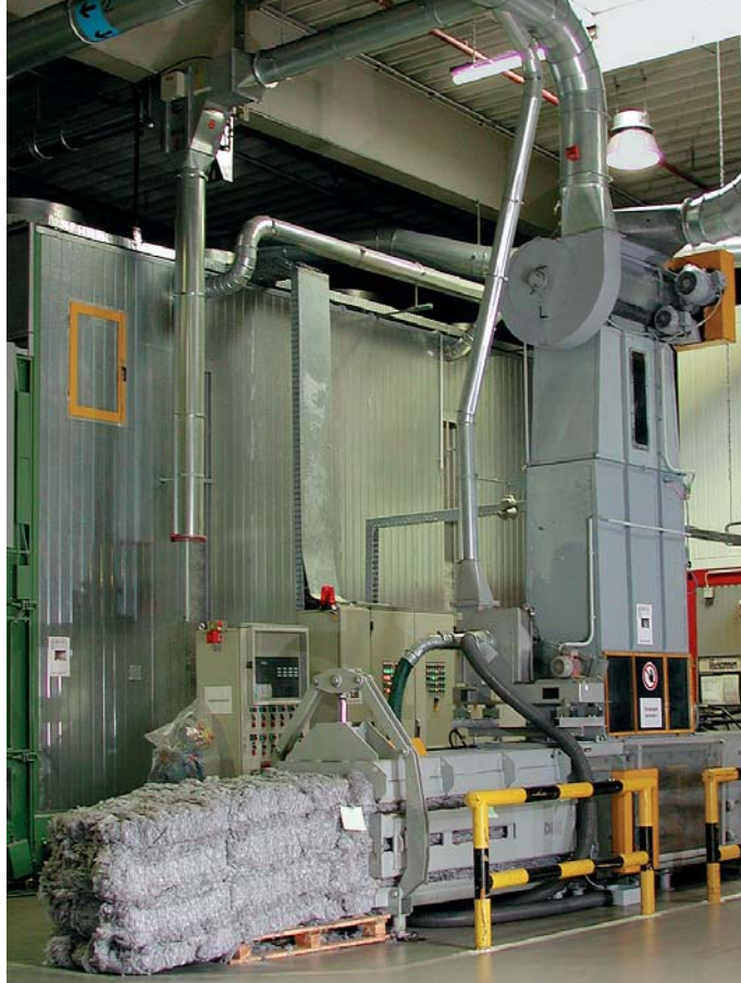
DIXI 50 SLK for the compacting of textile fibre in the insulating material production.
