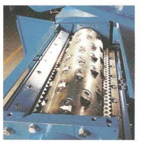
EZ 100 universal shredder with disposable cutting inserts which can be rapidly and individually replaced.
