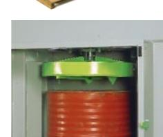
Large press ram: With venting spikes and guided on both sides.
