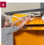
**1** Compact your waste and eject the finished bale. **2** Remove and store the bale until collection. 3 An efficient and silent ejecting system ensures easy handling of the compressed bale. 4 The strap rolls are easy to replace in front of the machine.
