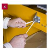
1 Compact your waste and eject the finished bale. 2 Remove and store the bale until collection. 3 The finished bale is ejected automatically by a safe two-hand operation. 4 A safe knife is mounted in front of the baler to help cutting straps.
