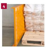
1 Compact your waste and eject the finished bale. 2 Remove and store the bale until collection. 3 Strap rolls are easy to replace in front of the machine. 4 Rows of barbs inside the chamber keep the waste material down.
