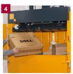
1 Compact your waste and eject the finished bale. 2 Remove and store the bales until collection. 3 Tying of straps through the press plate gives a compact and stable bale. 4 The wide filling opening ensures optimal loading of large boxes.
