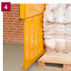
1 Compact your waste and eject the finished bale. 2 Remove and store the bale until collection. 3 With the vertical door you obtain an ergonomical working posture. 4 Rows of barbs inside the chamber keep the waste material down.
