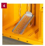
1 Compact your waste and eject the finished bale 2 Remove and store the bale until collection. 3 Strap rolls are easy to replace in front of the machine. 4 An efficient and silent ejecting system ensures easy handling of the compressed bale.
