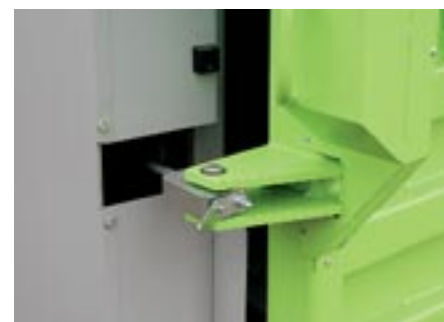
The hydraulic door opening mechanism
